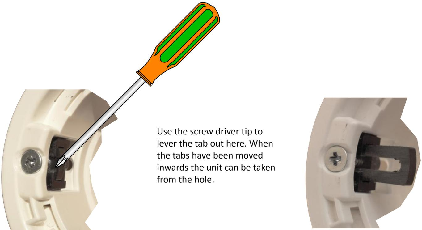
Use the screw driver tip to lever the tab out here. When the tabs have been moved inwards the unit can be taken from the hole.
