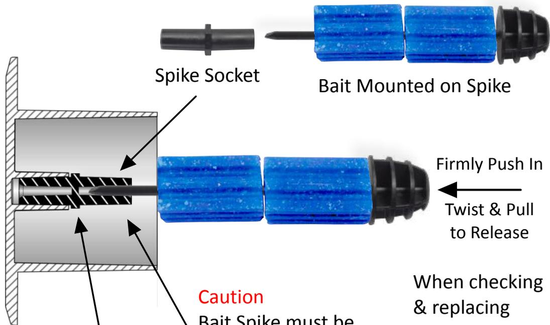
Spike Socket must be **tightly** inserted into the base unit at all times.
